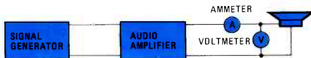
Fig. 5—HOW WOOFER ADMITTANCE was measured. Admittance is used as a diagnostic to determine several parameters.
